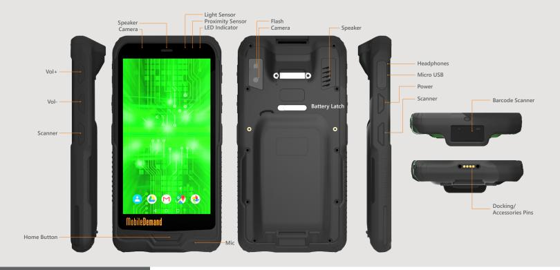
6" Sunlight Viewable Display MT8735b Quad Core Processor Ruggedized IP65 Sealed Wi-Fi
