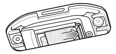
4. Push the SIM card into the SIM slot.
