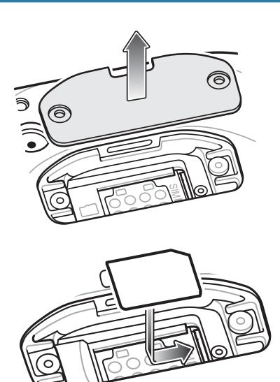
3. Align the SIM card with the SIM slot.
