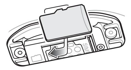
4. Push the microSD card into the SD card slot.
